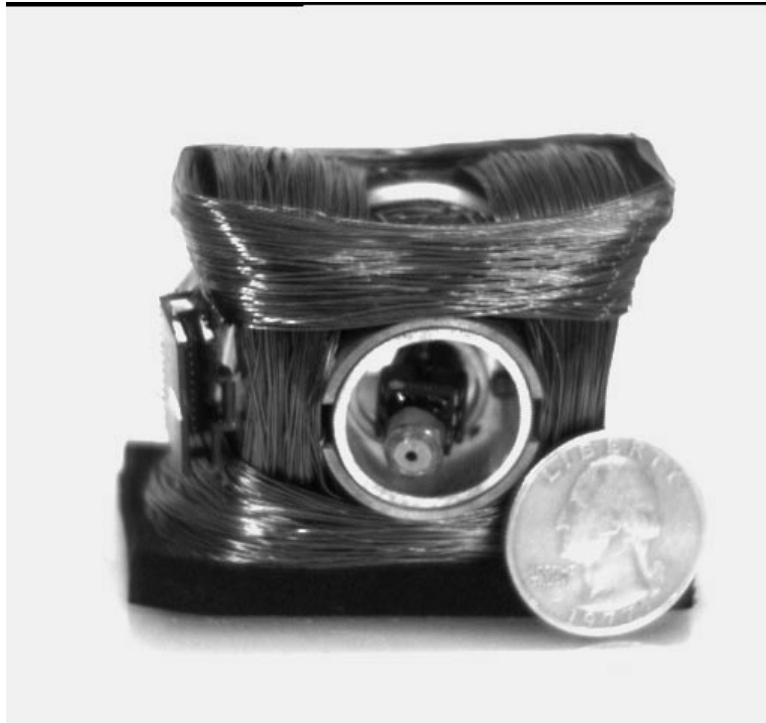
Figure 4.1: The Spherical Pointing Motor. At the center is a miniature camera consisting of a single CCD sensor chip and a lens assembly that fits on the rotor of this motor.
