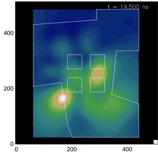
Fig. 6. The NBI detector measured the SRS in a NIF experiment performed on Dec. 4, 2009. This data is from a 30 degree quad at a time of 19.5 ns. The rectangles show the location of the 4 lenses. The other lines show the border of the NBI scatter plate. The SRS covers an area much larger than the lenses. (The image was normalized to use the full color table.)
