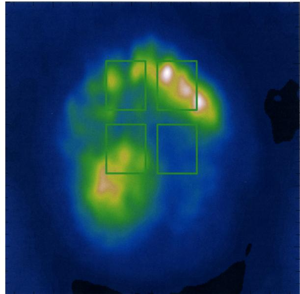
Fig. 8. This figure shows the SRS pattern from pF3D at the target chamber wall near the end of a burst (18.8 ps). The location of the brightest spots has shifted significantly towards the upper right relative to the peak of the burst. (The image is normalized to use the full color table.)
