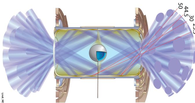
Fig. 1. The figure shows the laser beams entering the hohlraum through holes at both ends and propagating through the plasma until they reach the hohlraum wall. The hohlraum is a "can" used to trap and re-radiate the x-rays emitted by the hot interior walls of the hohlraum.
