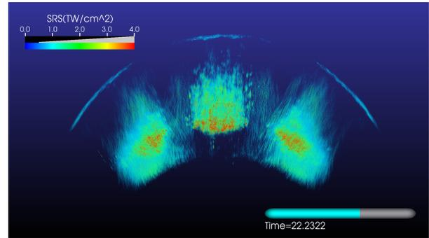
Fig. 5. The SRS comes in bursts. At this time, SRS is generated independently in each quad. Later in the burst, SRS is generated in the region where the quads overlap.
