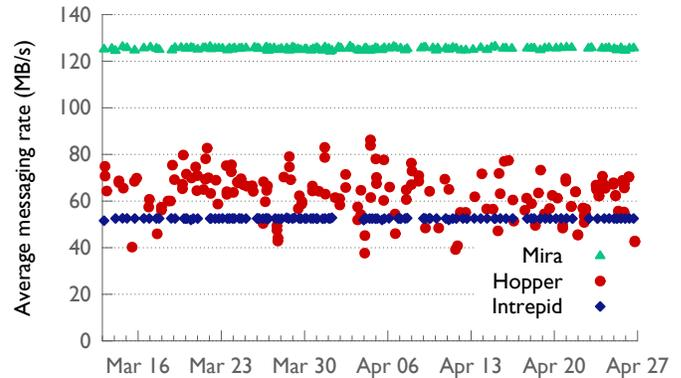
Fig. 4. Average messaging rates for pF3D batch jobs running on IBM Blue Gene/Q (Mira - green), a Cray XE6 (Hopper - red), and an IBM Blue Gene/P (Intrepid - blue). The slowest message rate on Hopper is half the fastest rate.
