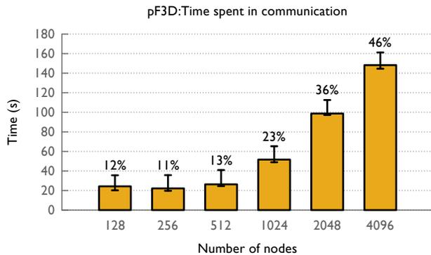
Figure 2: Average, minimum, and maximum time spent in communication by pF3D for weak scaling on Blue Gene/Q
