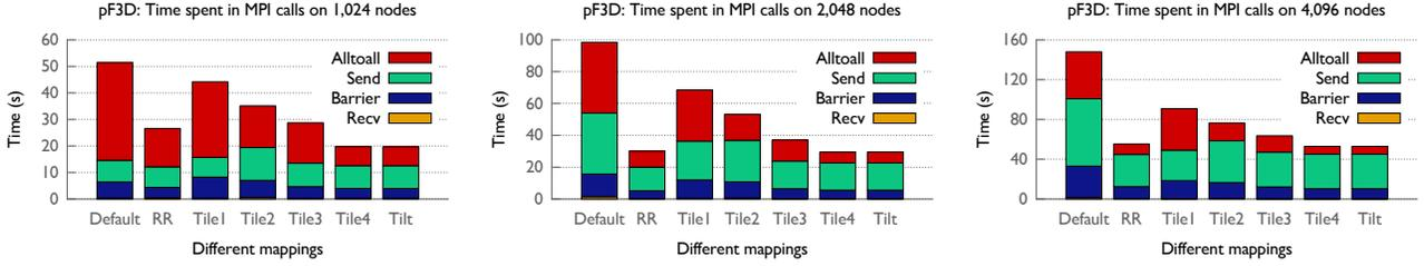
Figure 5: Reduction of time spent in different MPI routines by using various task mappings for pF3D running on 1,024, 2,048 and 4,096 nodes of Blue Gene/Q (Note: y-axis has a different range in each plot)
