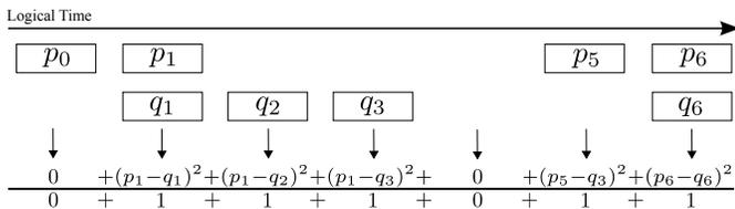
Fig. 4: Distance between two logical timelines with metrics  $p_i$ ,  $q_i$ . When both processes exhibit an event, we use the squared difference. When only one process exhibits an event, we use the difference between the event and a prior event if it exists.
