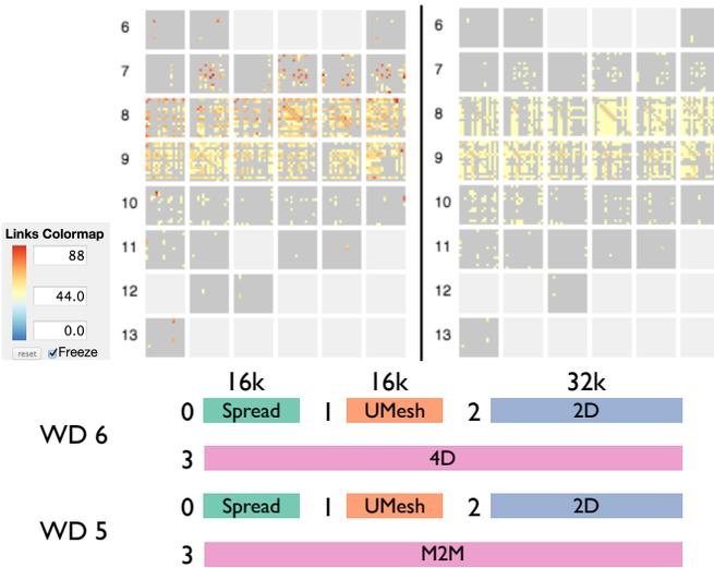
Figure 10. Max. traffic on green links for Job 1 (UMesh) is higher when situated near a communication-heavy job (4D Stencil) in WD 6 (left) than when situated near a communication-light job (Many-to-many) in WD5 (right).
