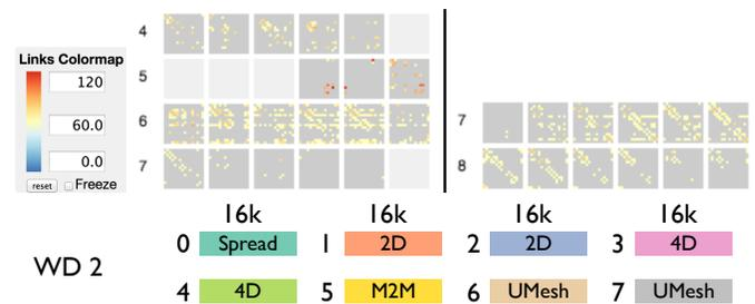
Figure 7. Traffic on green links attributed to Job 6 (left) and Job 7 (right) in WD 2. Both jobs represent UMesh running on 16k cores. Job 6 shares group 5 with a communication-heavy Job 4 (4D Stencil), which in turn leads to higher congestion (maximum traffic: 119.5 MB for Job 6 versus 72.4 MB for Job 7).
