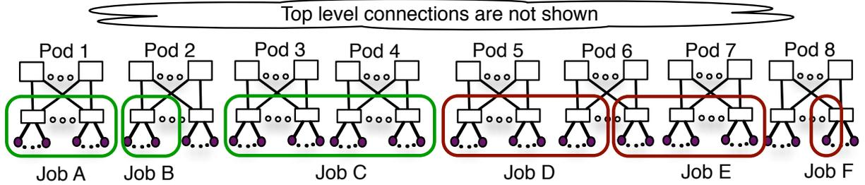
Figure 10: Partitioning a fat-tree: if each job is allocated either 1) all nodes connected to one or more switches in a single pod, or 2) all nodes connected to all switches in one or more pods, inter-job interference can be eliminated.
