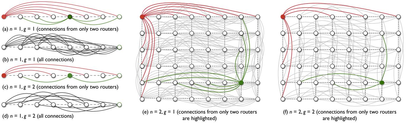
Figure 2: Construction of one- and two-dimensional express meshes with gap,  $g = 1$  and  $2$ . Connections that are inherited from  $n$ -dimensional mesh are shown as dashed straight lines; new connections added are shown as solid curved lines.
