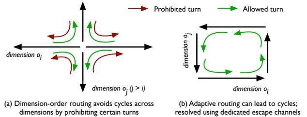
Figure 4: Deadlock freedom across dimensions: adaptive routing relies on escape channels using dimension-order routing to break deadlocks [10].
