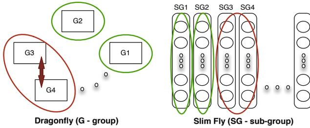
Figure 11: Partitioning dragonfly and Slim Fly: only if each individual job is contained within distinct groups and sub-groups respectively, inter-job interference can be avoided.
