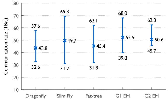
Figure 7: Comparing performance on different networks using 30 different multi-job workloads. Values shown are minimum, median, and maximum across different workloads.
