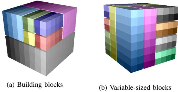
Figure 12: Partitioning express mesh: convex shape allocations eliminate inter-job interference (each color represents a job allocation; different shades used to show individual routers).
