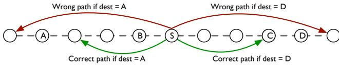
Figure 3: Routing within a dimension: messages always travel toward the destination, but do not use additional links to go beyond the destination.
