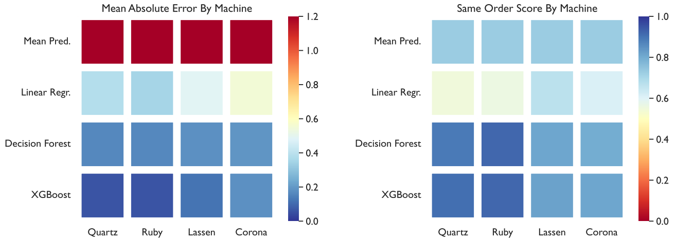
Fig. 3. The MAE (left) and SOS (right) of each model when predicting using counters data from one particular machine. For instance, the bottom right of the left visualization represents the MAE when predicting relative performance vectors with XGBoost and counters data from Corona. Lower MAE, or more blue, is better, and higher SOS, or more blue, is better.
