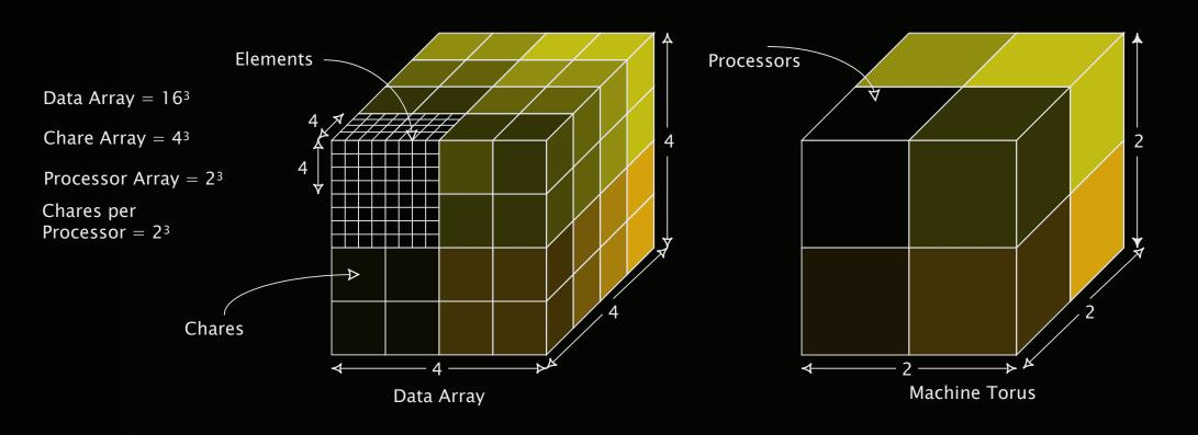
The 3D data array was divided into cubes and each cube was assigned to one Charm++ Virtual Processor (VP). The runtime does a default placement of the VPs. Round-robin and topology-aware mapping schemes were compared with the default scheme and the results are presented below:
