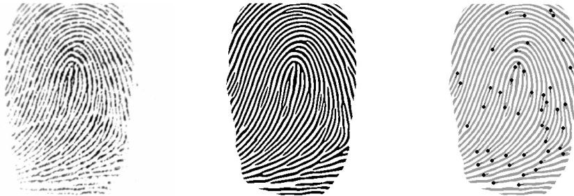
Figure 2.3: Feature Extraction Process: (a) original image, (b) after edge detection, (c) including feature points
