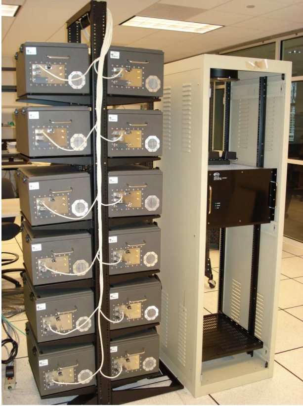
Fig. 1. Assembly and connection of the shielded enclosures and RF switch.
