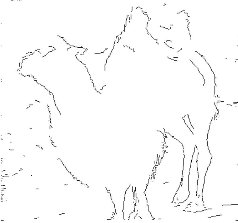
Figure 14: Canny edge detector, best results (thresh=[.1, .35], \sigma = 3.5 )
