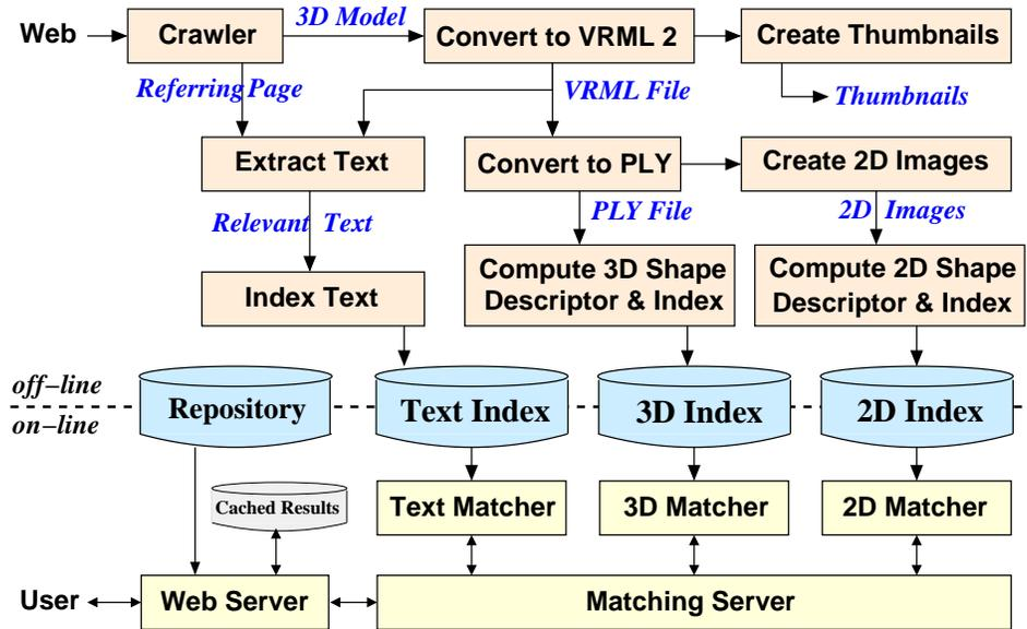
Fig. 11. Flow of data through the search engine. The data shown in blue text is stored in the repository.
