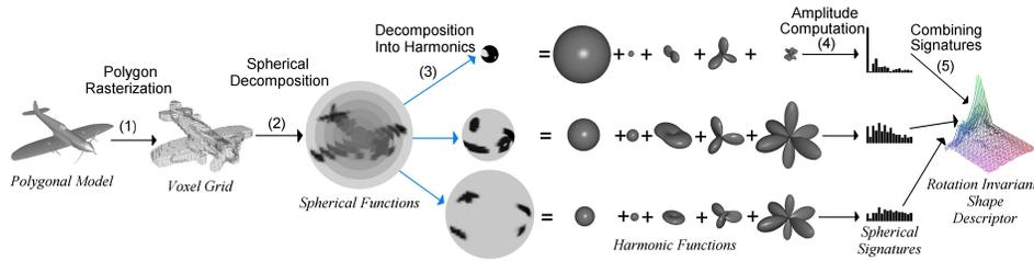
Fig. 4. Computing our spherical harmonics shape descriptor.
