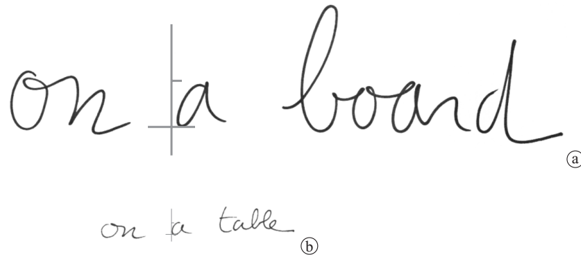
Figure 11: Handwriting on a board. Because users must use their arm to form the letter shapes while writing on a vertical board, they naturally write bigger (around 96 points) (a) than when they write on a table (around 24 points) (b) . The rules indicate height for a lower-case letter, depth for a descender (such as y), and leading, based on 96-point and 24-point Times Roman, respectively.
