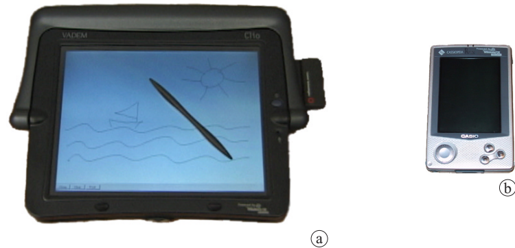
Figure 54: PDA used in the experiment. 3 Clio 1000 (a) and 3 Cassiopeia (b) were used as digital sketch pad. The Clio is shown running the simple sketching application.
