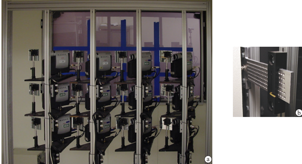
Figure 20: Overview of the final projector array setup. The system skeleton shown in (a) is built out of extruded aluminum, and each projector is mounted on an alignment platform (shown in more detail in Figure 21). In the background, one can see the masking tape (blue bands) used to mask the outermost 16 pixels of each tile (see Section 4.2.2). The pieces of tape adhere to a large sheet of acrylic held in position by four mounting points such as the one shown in (b). The pattern of holes in a mounting point is designed so that the distance between the masks and the screen can be adjusted by 1-mm increments.
