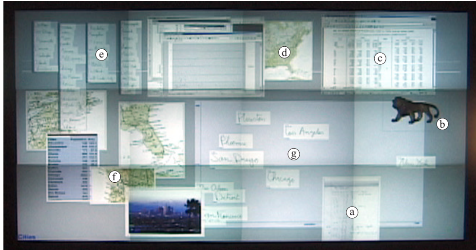
Figure 46: A typical PostBrainstorm screen. The user has accumulated content from various sources (counter-clockwise from the bottom right): a scan of a sketch (a), a 3D model of a lion (b), a VNC connection (c), an annotated map of the USA (d), several lists of handwritten material (e), several snapshots (f), and in the center a scatter plot container (g).
