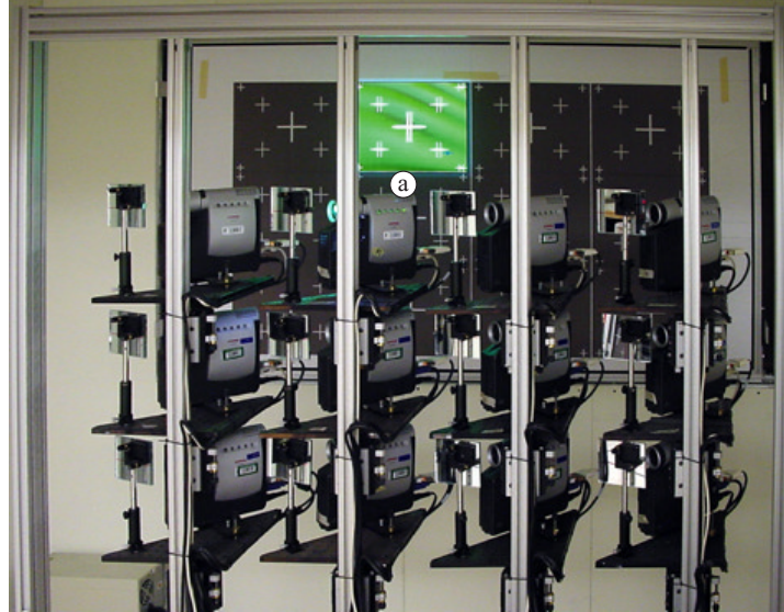
Figure 23: The reference alignment pattern in place. The pattern is printed on a large piece of foamcore and its distance from the screen can be adjusted using the mechanism shown Figure 20a. We show one projector projecting a set of vertical green strips and the resulting moiré pattern can be seen (a). The crosshairs superimposed on the reference pattern provide a reference to detect parasite rotations and translations.
