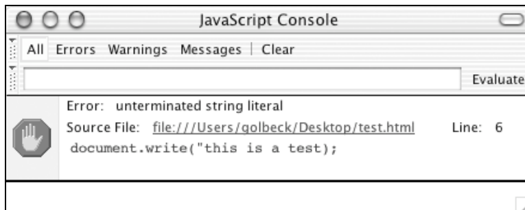
Figure 17.2: The JavaScript console showing an error on Line 6 of this test file.
