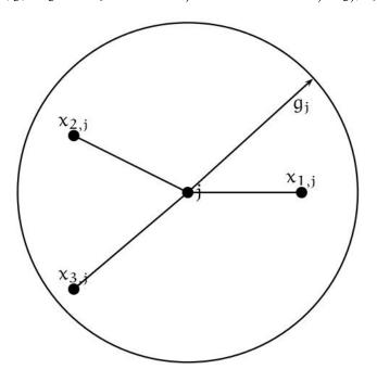
For a client  $j \in D$  sort all the  $i \in F$  facilities according to  $c_{ij}$ . Let  $c_{\pi(1),j} \leq c_{\pi(2),j} \leq \ldots \leq c_{\pi(f),j}$  be the sorted order.
