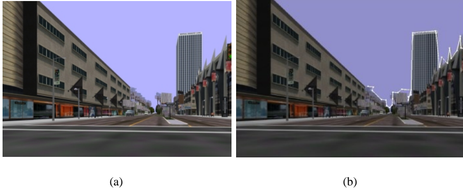
Fig. 7. (a) Original image from a virtual reality system. (b) World model (white lines) projected into this image using the pose computed by SoftPOSIT.
