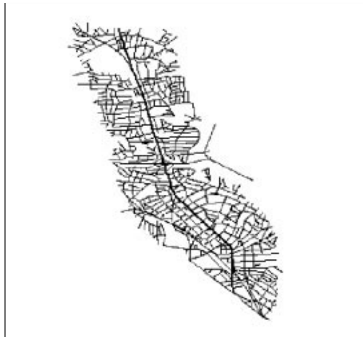
Figure 2: Example of spatial join. Map of Silver Spring showing line segments corresponding to Georgia Ave (thick line) and all line segments of streets within one mile of Georgia Ave (thin lines).
