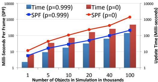
Figure 15: Figure shows the milliseconds to render a frame and the time in milliseconds spent per frame to update the data structure for varying sizes of the simulations
