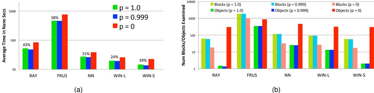
Figure 14: (a) Query times, using a log scale, for operations using the loose quadtree for values of  $p = 0$  (the MX-CIF quadtree),  $p = 0.999$ , and  $p = 1$  where  $p = 0.999$  performs best as indicated with the percent improvement over the MX-CIF quadtree. (b) The average number of blocks and objects visited by the query
