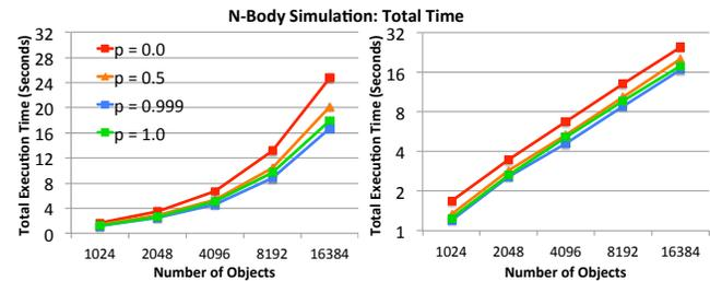
Figure 12: CPU execution time for insertions in the N-body simulation using a normal scale (left) and a log scale (right).
