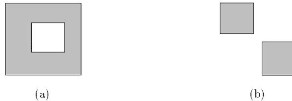
**Fig. 8.** Some polygons with holes (a) or having more than one connected components (b) cannot be coarsened with the “moving faces” approach.
