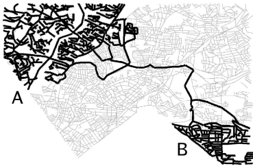
Figure 2: The 30,000 shortest paths between two subsets A, B of vertices in a road network of Silver Spring, MD pass through a single common vertex
