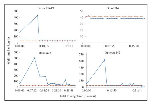
Figure 5. Optimal parameter search across multiple platforms. Solid blue line represents performance results discovered over time. Dashed and dotted lines represent the min, max, and average of 10 control runs.
