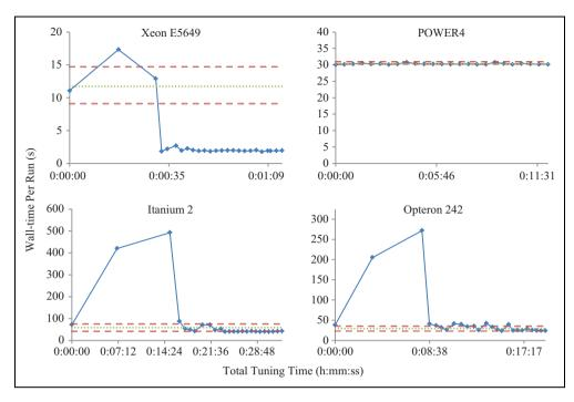
Figure 3. Tuning quicksort across multiple platforms. Solid blue line represents performance results discovered over time. Dashed and dotted lines represent the min, max, and average of 10 control runs.
