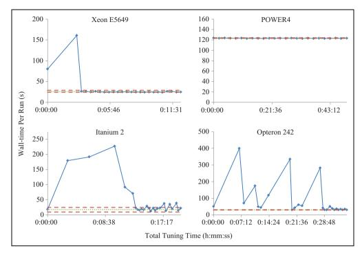
Figure 4. Tuning STREAM across multiple platforms. Solid blue line represents performance results discovered over time. Dashed and dotted lines represent the min, max, and average of 10 control runs.
