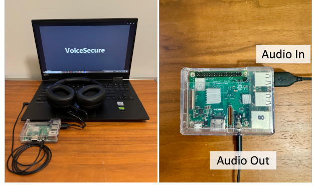
Figure 8: VoiceSecure module: (left) connected to commercial headphones during an audio call; (right) close-up of the module showing two audio ports.
