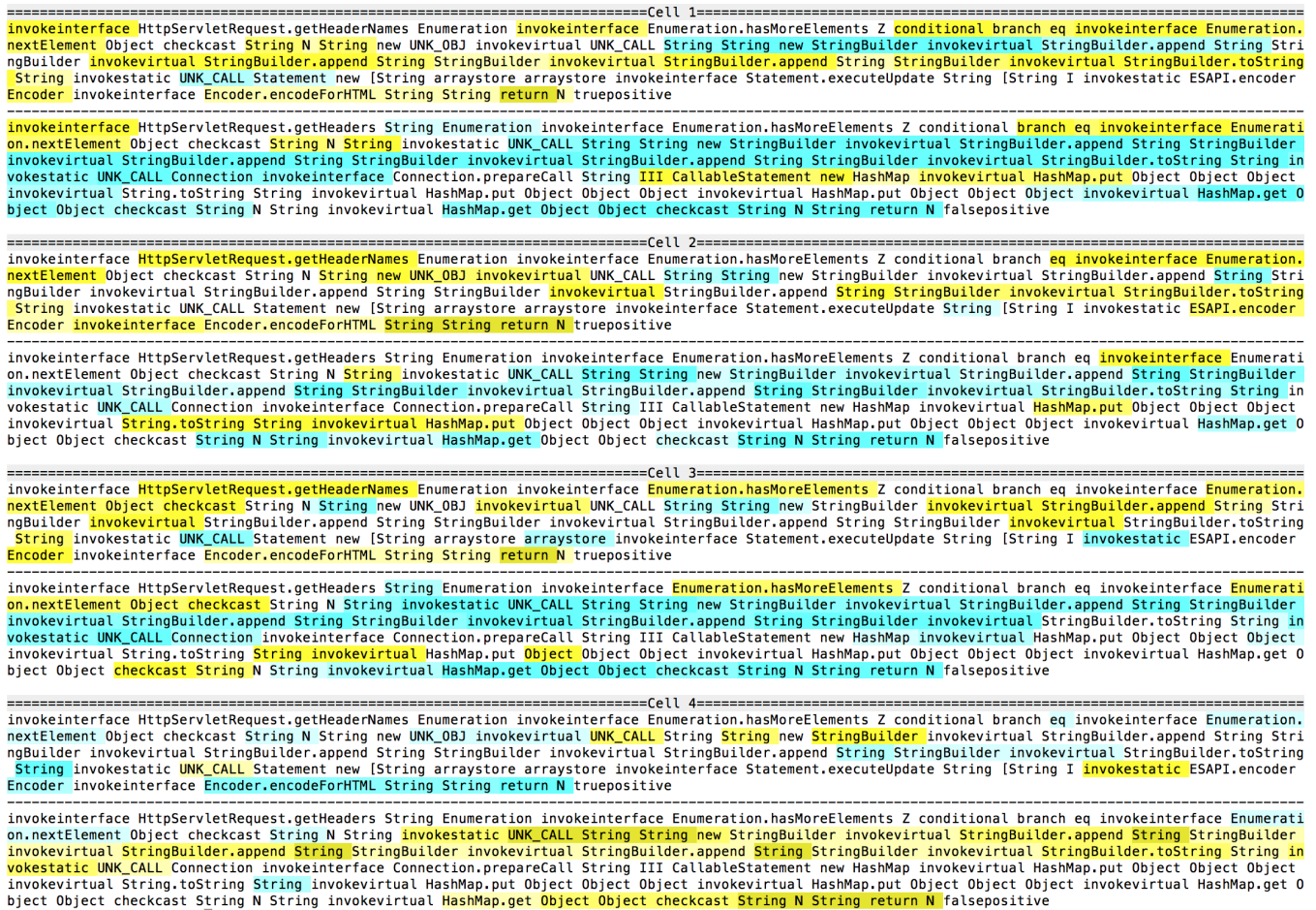
Figure 4. LSTM color map for two correctly classified slices. First slice is a true positive and second slice is the false positive in Figure 3. Cyan, yellow, and white background mean positive, negative and under threshold ( \pm 0.35 ) output value respectively. There is only one tint of white, but for cyan and yellow, the darker the background the larger the output is (in magnitude).
