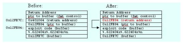
Thus, by not following the exact specification, programmers can allow hackers to overwrite values in memory and execute arbitrary code. While the improper usage of the format function family is widespread, finding vulnerable programs is also relatively easy.
