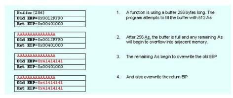
malicious code. Also, instead of overwriting the return EIP (where the program will execute next) with random bytes, the exploit will overwrite EIP with the address to the buffer which is now filled with malicious code. This causes the execution path to change and causes the program to execute injected malicious code.
