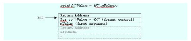
However, by using printf incorrectly, the stack will appear differently since one does not push on the argument list and only the format control.
