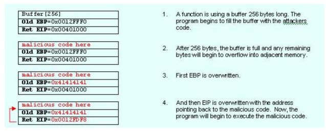
While the above example demonstrates a classic stack-based (first generation) buffer overflow, there are variations. The exploit utilized by CodeRed was a first generation buffer overflow that is more complex and is described below.
