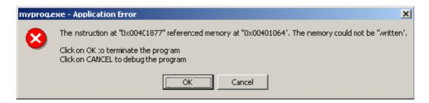
However, this demonstrates one can write to memory. With this ability, one would actually wish to overwrite a return pointer (as in buffer overflows) redirecting the execution path to injected code. Examining the stack more fully, one determines in the example program, the stack appears as follows:
