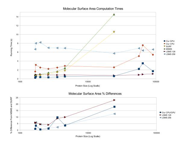
Fig. 3. Surface area computation times and percent differences for proteins of different sizes using several different algorithms. Data is from table 1. Protein size is given in RBFs, which is equal to the number of atoms listed in the PDB file. For MSMS and SURF, data is not available for the larger proteins since these programs were unable to compute the area for proteins of that size. Percent differences are given as absolute magnitudes.
