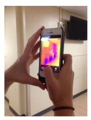
**Figure 1:** Thermal cameras have recently been introduced into the smartphone ecosystem and provide an opportunity for users to detect, identify, and assess thermal defects in buildings. Here, a FLIR One [21] (connected to an iPhone 5s) is used by one of our pilot study participants to assess a hallway in a building on the University of Maryland's campus.
