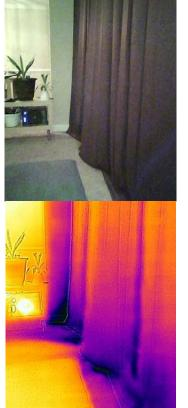
**Figure 6:** A participant in our pilot study described using a thermal camera to measure temperature exchange in her apartment resulting from the floor-to-ceiling windows (behind the curtains). The pilot participant took photographs over several hours and deduced that the rate of thermal exchange increased as a function of the difference between the internal and external temperatures; this experiment was designed to confirm a previous comfort concern.
