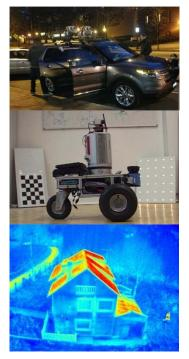
**Figure 4:** Examples of thermal data collection techniques from research literature and in industry: (a) Essess Inc.'s Google Street View like cars with mounted thermal cameras [12]; (b) Irma3D indoor thermal mapper robot [15]; (c) residential data from a UAV with a mounted thermal camera [11].
