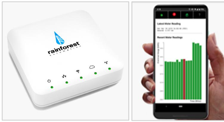
Fig 2: Our prototype system relies on the Rainforest Automation EAGLE-200 home energy hub for access to real-time energy data (left) and we are designing real-time energy displays and learning modules that support the KYEN program's education goals through a collaboration with the METER team at The University of Oxford (right).
