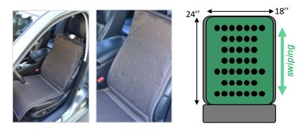
Fig. 2. Seat configuration covering a back space of 12x18 inch grid, able to produce a variety of haptic stimulation patterns.
