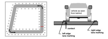
Fig. 4. (*Left*) Driving course. (*Right*) Lane departure as described by the SAE Standards for Operational Definitions of Driving Performance Measures [28].
