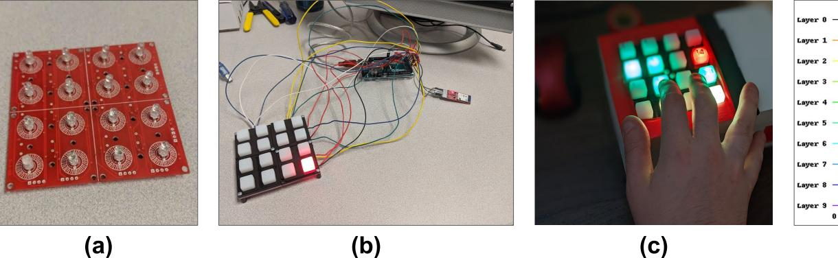
**Figure:** Our custom remote control was constructed from a 4x4 grid of multicolor LED and soft button panel (a), connected to an Arduino microcontroller and Bluetooth dongle (b), and then enclosed in a 3D printed case (c). The controller pairs with an audio player application created in Unity3D. Interactions with the remote are logged and can be output to create visualizations of the interactions that users have with the device and music (d).
