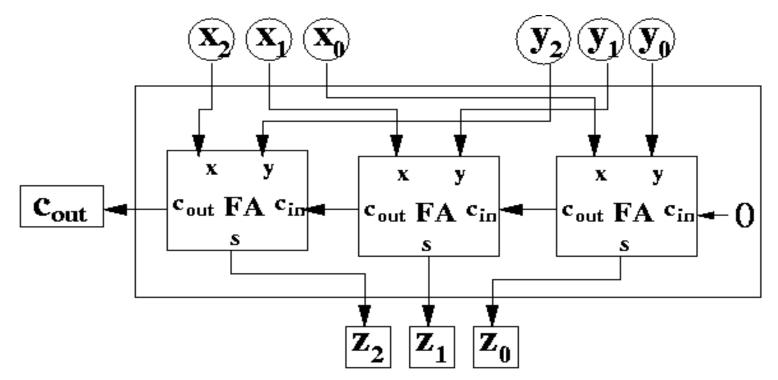
Notice that 0 is hard-wired as carry-in for rightmost full adder (could have used half adder)
