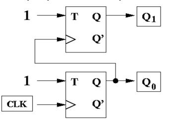
What will be the period of the second flip-flop output  $Q_1$ ? If we keep repeating this N times, the period of the Nth output will be  $2^{N}t$ How does this help build a counter?
