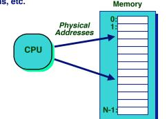
Addresses generated by the CPU correspond directly to bytes in physical memory
