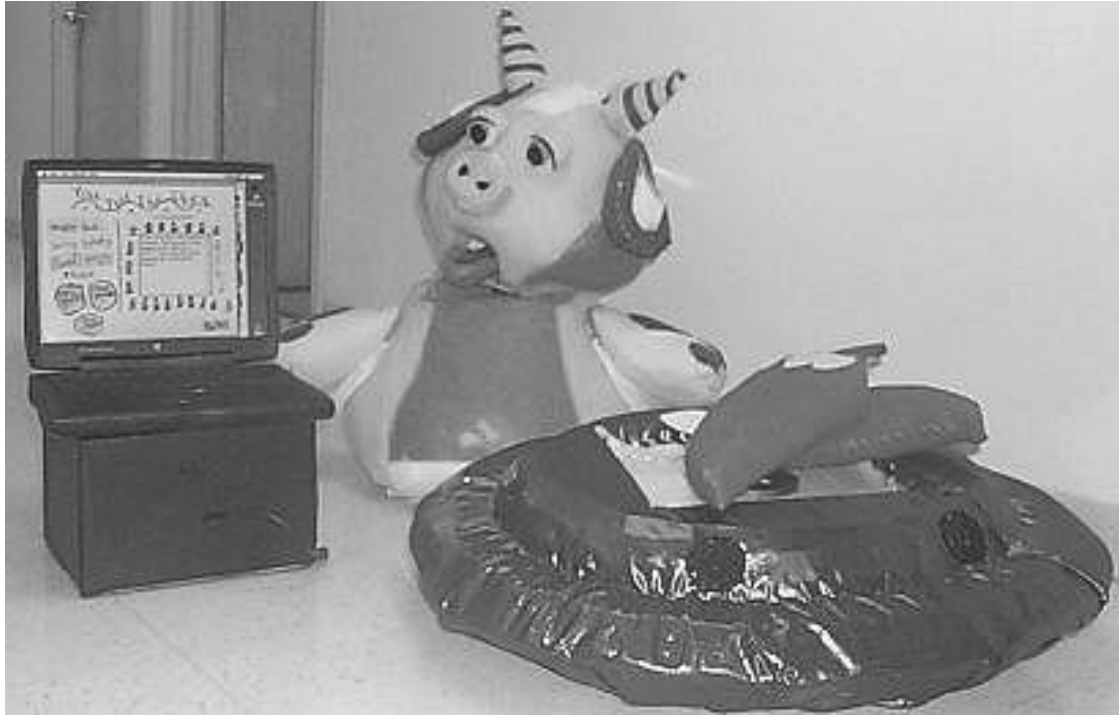
Figure 4.1: PETS. On the left is a computer displaying the MyPETS software. In the middle is the PETS robot decorated with paws, a pig's snout, horns, and floppy ears. To the right is a flying saucer for PETS to ride on. On top of the flying saucer are an optional pair of wings.
