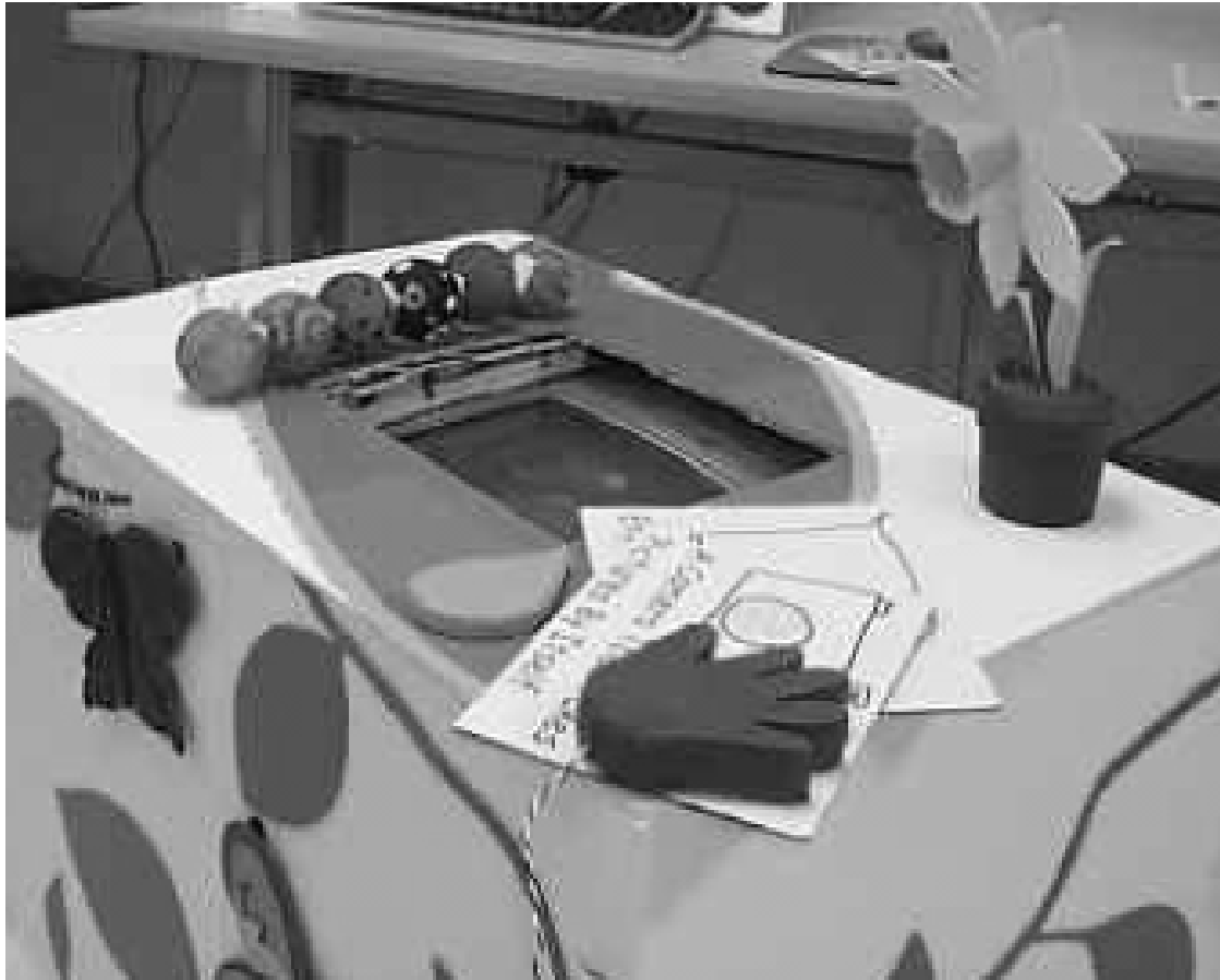
Figure 5.17: A conceptual Storybox. To the left was a StoryWorm made from individual worm segments. The head of a worm would “remember” a story. Each segment “remembered” a line (or interaction rule) in the story. The flower was a microphone for children to record sounds. The monitor in the center would display the different lines of a story. Each line corresponded to a worm segment next to it.
