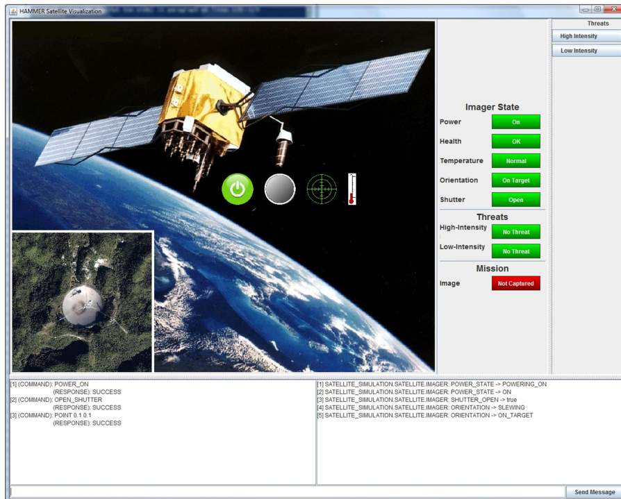
Figure 6. The HAMMER satellite demonstration display gives the user control over solar events and shows the status of various satellite components, sensors, and mission goals.
