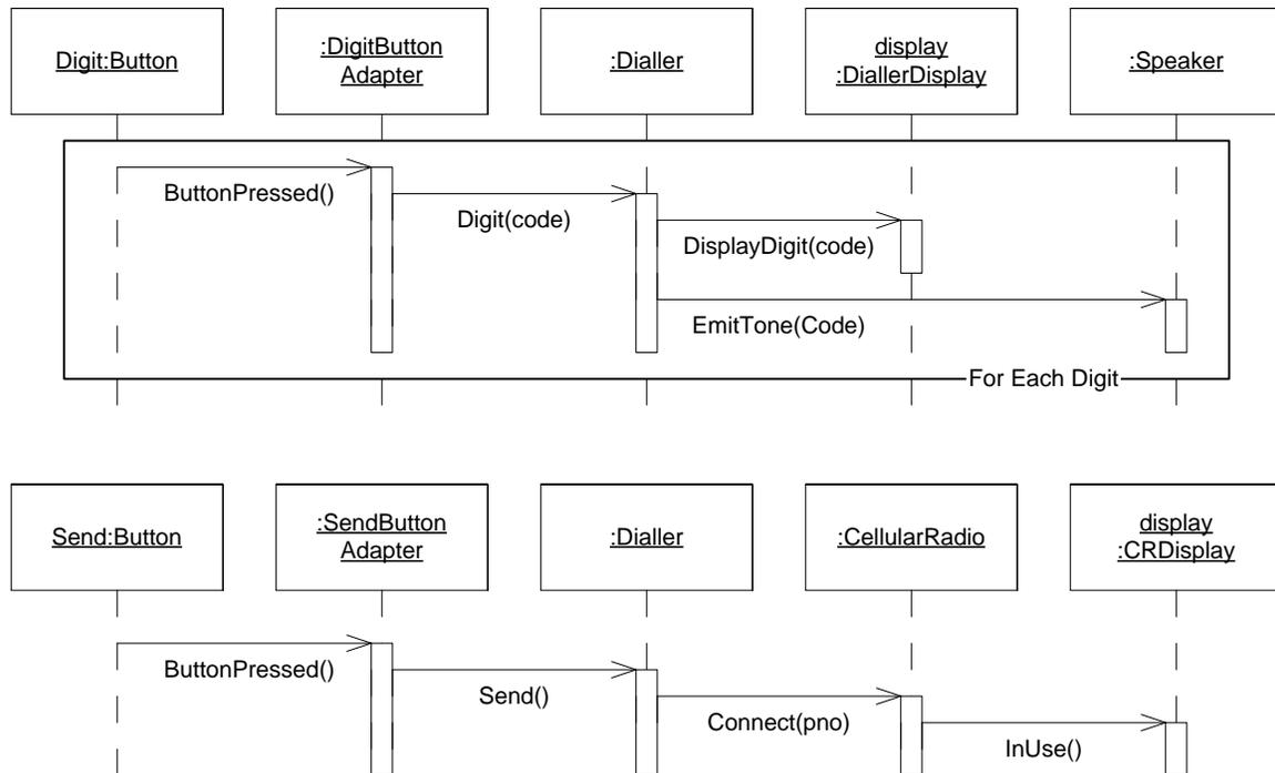
**Figure 2: Sequence Diagram of Cellular Phone.**
