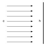
Assume for the moment that the surface is 1 unit deep into the page, so the area is h\*1 = h. Now the irradiance is c/h, so the incoming radiant energy is spread over the area h (irradiance is watts over meter squared, or energy over area).
