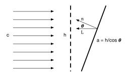
Here **a** is the new area over which the incoming radiant energy is spread. **a** increases as the reciprocal of the cos of the tilt angle. We have only a 2D diagram, so **a** is represented here by the length of a line and not properly area, but since we assumed the surface is 1 unit deep into the page and is not tilting into the page, the area increases proportionally to the new length.
