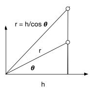
If we reorient our diagram to consider the light from a beam of radiant energy **c** impinging on a surface **h** high we get this diagram when the surface is perpendicular to the incoming light.
