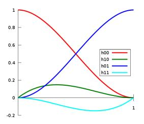
The way to look at this is, each of the curves weight the input data points, so the red curve (h00) represents the proportion of P0 that contributes to the output point.
