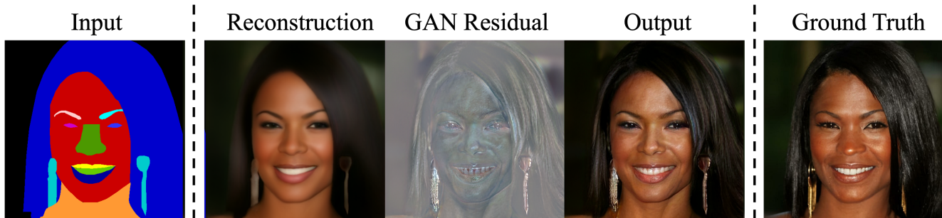
Figure 1. We decouple the optimization of reconstruction and adversarial losses by synthesizing an image as a combination of its reconstruction (low-frequency) and GAN residual (high-frequency) components. The GAN residual adds realistic fine details while avoiding the pixel-wise penalty imposed by reconstruction losses.
