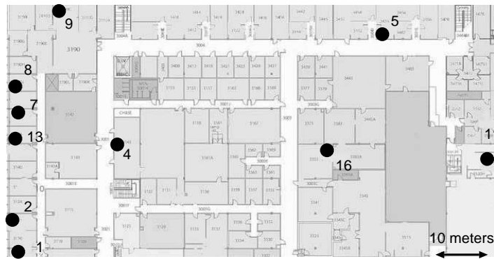
Fig. 12. Partial floorplan for the Emulab wireless testbed. Nodes 1 and 9 cannot directly communicate, and all the other node pairs can talk to each other.
