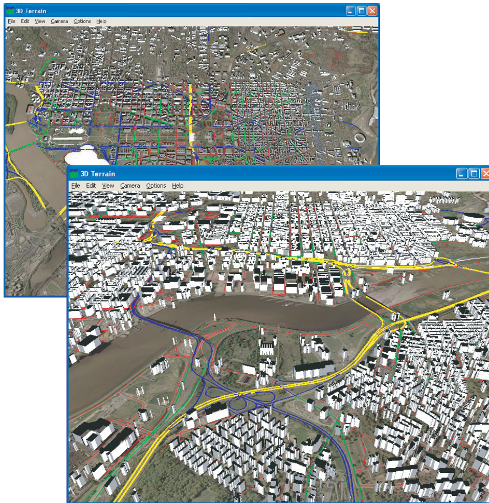
FIGURE 2 User flies high above city. Varying levels of detail can be seen, depending on height of observer. Accident locations can be highlighted with different colors or beams of light.
