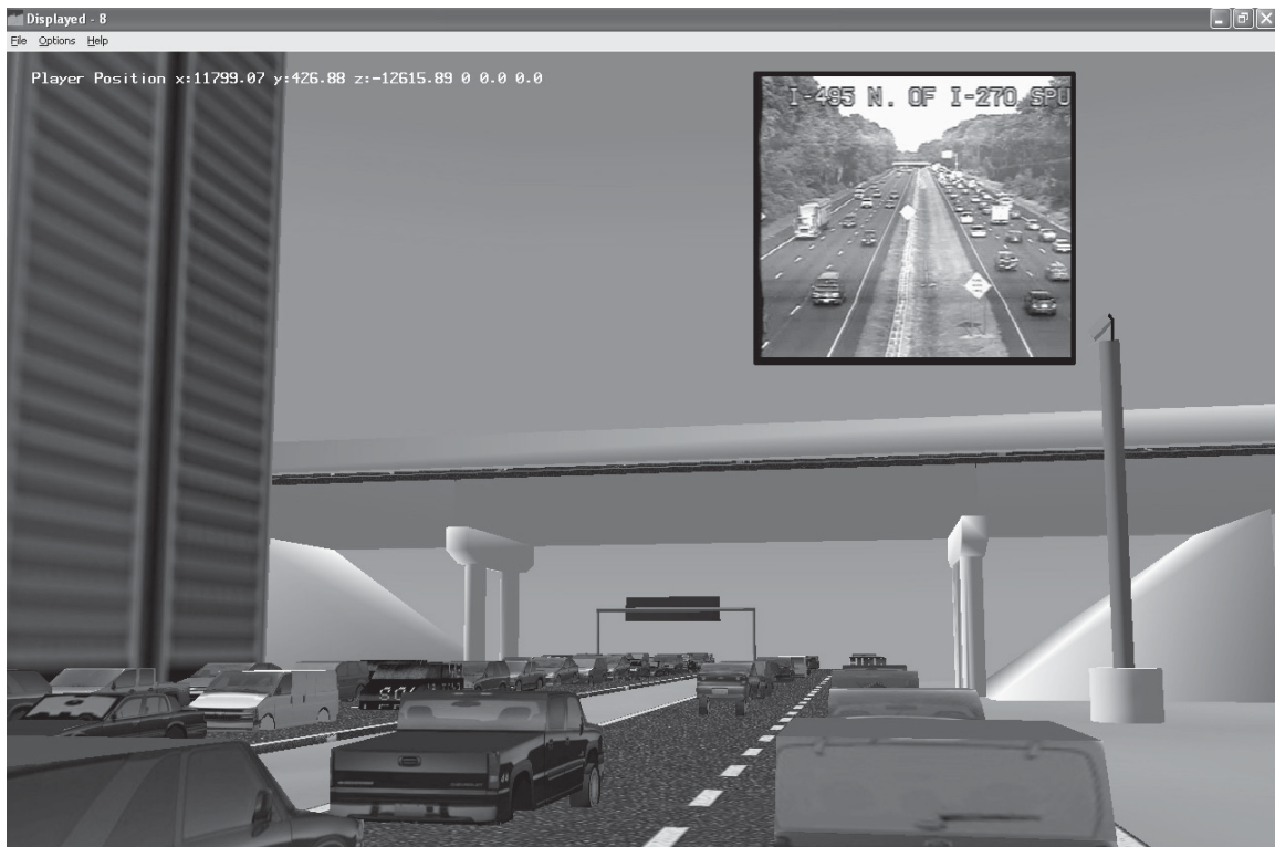
FIGURE 9 Dynamic 4-D rendering of area in Maryland with real-time CCTV video feed and traffic embedded in model.
