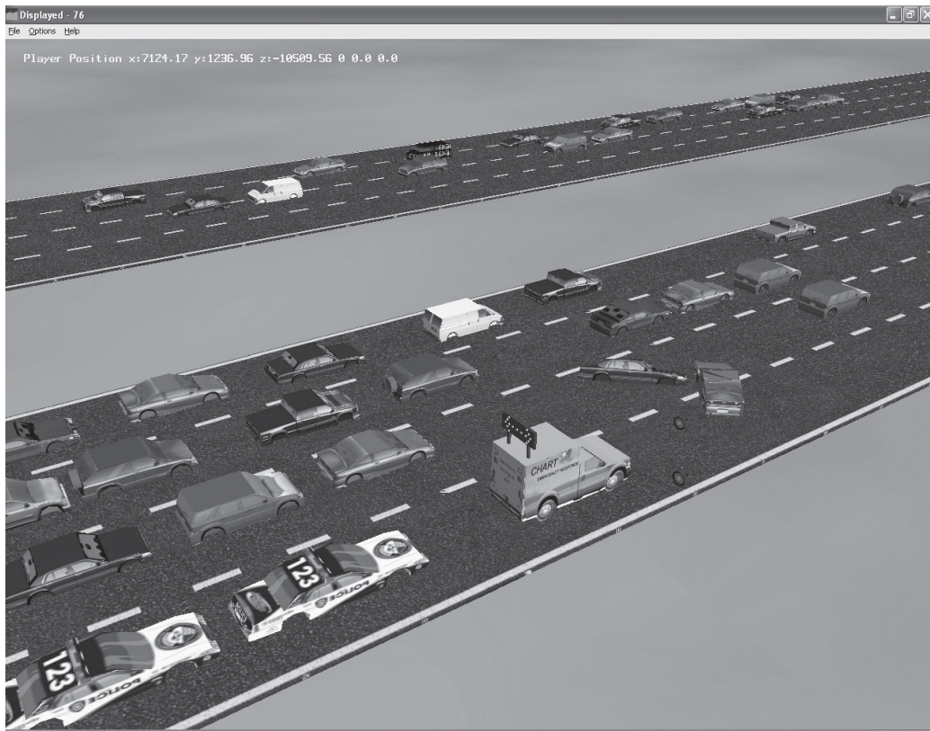
FIGURE 7 Dynamic 4-D rendering of two-vehicle accident blocking two lanes of traffic with three responding vehicles.
