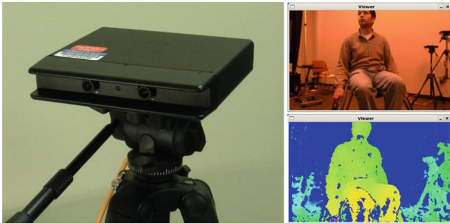
**Fig. 1** *Left:* A TYZX G2 stereo camera with onboard CPU and networking. *Right:* An example of the color and depth images produced by the G2 camera
