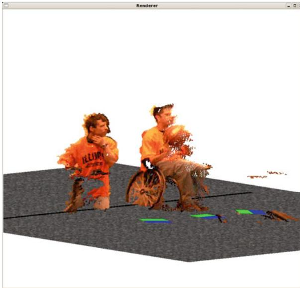
**Fig. 2** An example of the 3D reconstruction produced by the TYZX stereo cameras overlaid on top of a virtual floor
