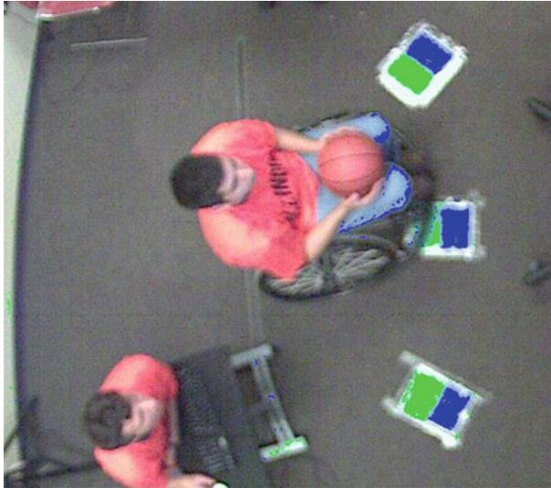
**Fig. 4** The floor markers observed from a ceiling mounted camera. Each pixel in the image is thresholded to separately find the bluest and greenest pixels in order to identify the markers. These pixels are then clustered in pairs to find the two halves of the marker. In the image above the marker pixels are replaced with *pure blue* (0, 0, 255) and *pure green* (0, 255, 0) (Color figure online)
