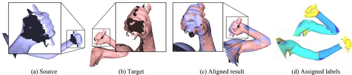
**Figure 8:** Registration for an arm dataset pair. The source mesh (a) is aligned to the target mesh (b). The hand region is missing a significant amount of data in both meshes, but after alignment the surface of the hand is completed nicely (c). The assigned labels are shown in (d) for the source (bottom) and the target (top), and corresponding parts have the same label assignment. Also, the segmentation naturally corresponds to the different parts of the arm.
