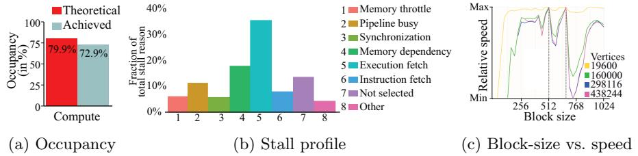
Fig. 10: Various performance profiles: (a) Occupancy metrics for the *Fusion 2* step with the best launch configuration, (b) relative stall profile for the final, most optimized implementation, and (c) impact of the block-size in the launch profile on performance
