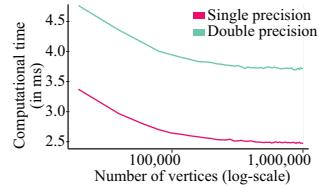
Fig. 12: Performance comparison of single and double-precision. Time per iteration per 1000 vertices of the mesh
