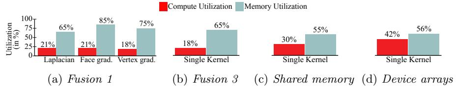
Fig. 9: Compute and memory unit usage for various optimization steps
