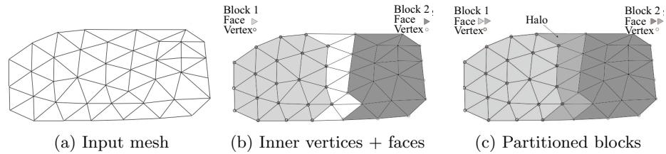
Fig. 6: Partitioning a mesh into two blocks
