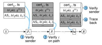
Figure 1: Ensuring the source ISP verifies certificates and enforcing that certificate holders compute valid signatures. Shaded regions represent pieces not verified at the next hop. A firewall operating on the receiver's behalf filters incoming traffic; the firewall may be colocated with the receiver or protect an access link.
