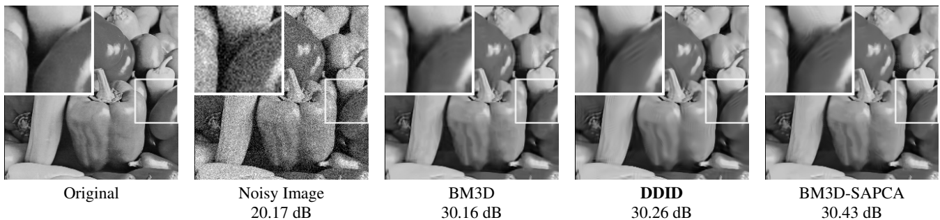
Fig. 6: Artifact comparison of DDID, BM3D, and BM3D-SAPCA. Misclassification of noise as signal due to accidentally regular patterns is acceptable and is to be expected. BM3D produces a smooth result, but this would fail in other occasions where the pattern would be a signal.
