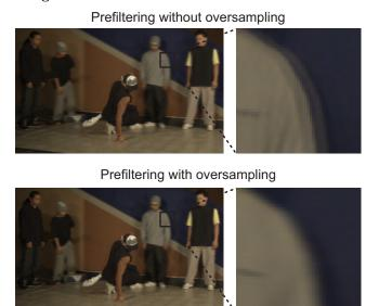
Figure 5: Comparison of pre-filtering with and without oversampling. Pre-filtering without oversampling leads to aliasing problems appearing as ghosting artifacts, shown at the top. Oversampling avoids these problems as shown at the bottom.
