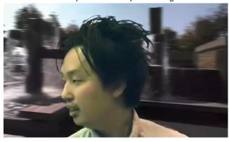
Figure 9: Comparison of compressed frames of a video sequence with and without pre-filtering. The images show simulated views of a multi-view 3D display. The version without pre-filtering at the top shows stronger blocking artifacts than the version with pre-filtering at the bottom. In addition, pre-filtering avoids ghosting artifacts, which appear without pre-filtering in the background in the top image.
