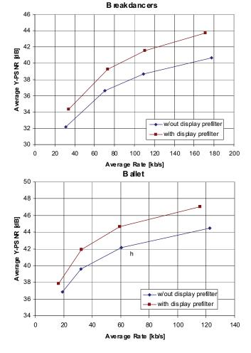
Figure 8: Comparison of RD curves for breakdancer and ballet sequences with and without pre-filtering.
