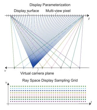
Figure 1: We illustrate the parameterization of a multi-view display at the top, and the corresponding ray-space sampling grid at the bottom.
