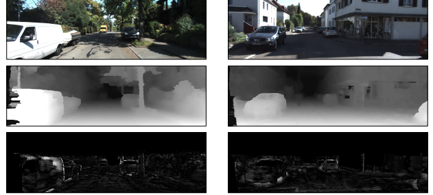
Figure 3. Examples results from the KITTI dataset. First row left image, middle row our final disparity and last row shows the errors clamped to 5.
