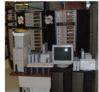
Beowulf computer cluster (Borg, 52- node cluster used by McGill University Image/Info from Wikipedia )
