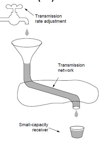
A fast network feeding a low-capacity receiver → flow control is needed
