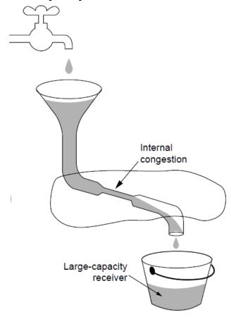
A slow network feeding a high-capacity receiver  $\rightarrow$  congestion control is needed
